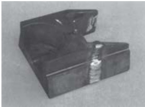
Fig. 34 Guide block of grey cast iron GG 25 for eccentric press. Combined welding of broken part, alternatively with NC-100 and NC-50 2.5 and 3.25 mm diam.
