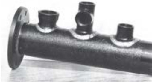
Fig. 33 Centrifugally cast pipe of ductile cast iron with welded flange and branches; an application for house connections of gas and water supplies as well as for intake shafts.
